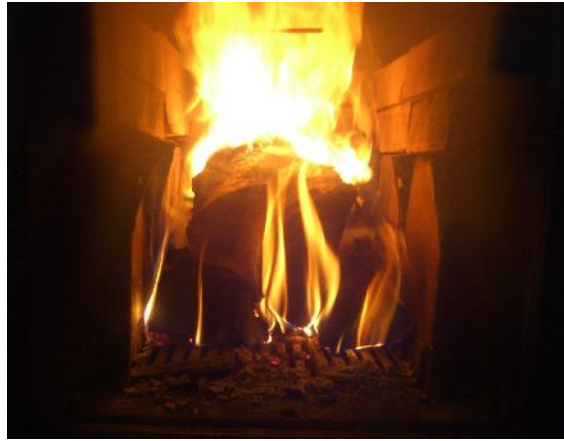
Figure 14. Number of tests at certain primary/secondary air ratio as a function of CO-emission on left (a), the flame structure in using secondary air on right (b).
