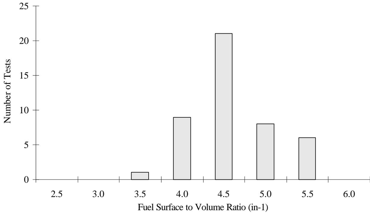
Figure 4. Distribution of average fuel sizing ratio for 45 masonry heater tests.
