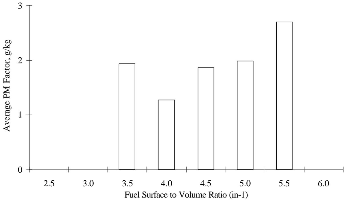
Figure 5. Distribution of PM emission factor by fuel sizing ratio for 46 masonry heater tests.
