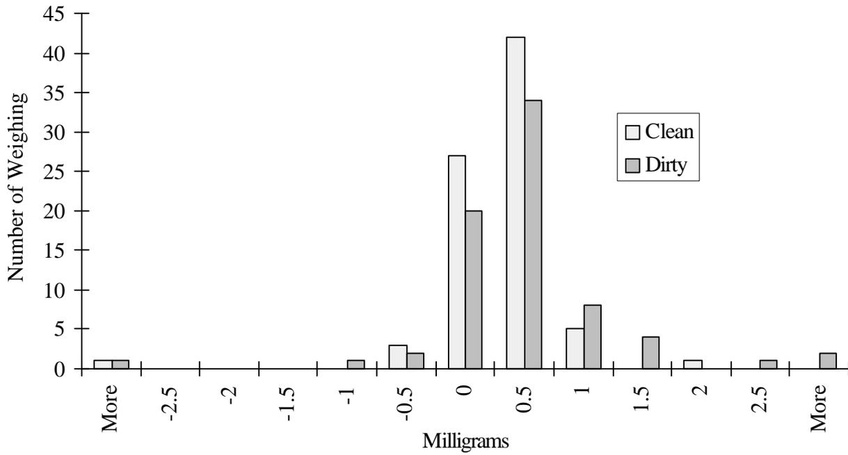
Figure 2. Filter weight discrepancies between batch and individual weights.
