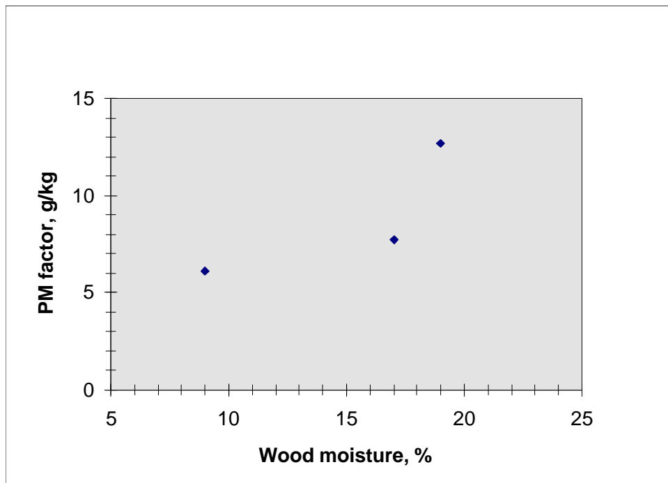
Figure 4. Correlation between PM factor and wood moisture for Buckley Rumford fireplace
