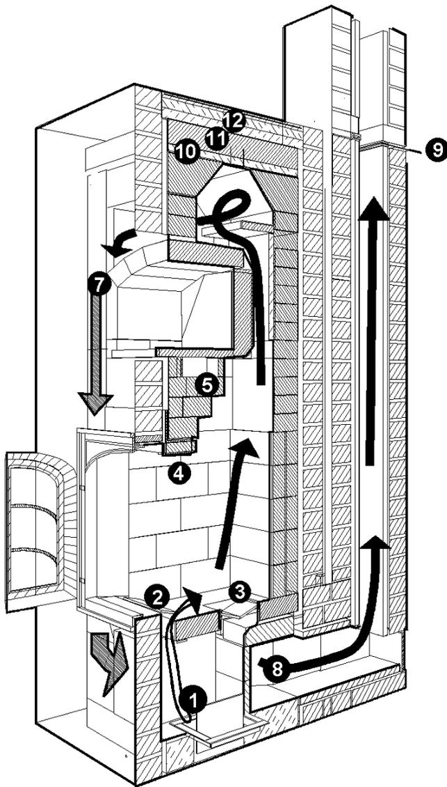
1. Insulating Base Slab with Outside Air Damper
