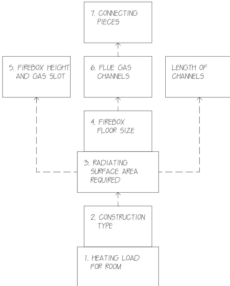
Figure 4. Construction sequence for Grundofen system
