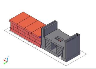
The bench is capped off with 12"x24" firebrick slabs, 2.5" or 3" thick.
