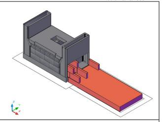
There is a cap brick inside the base channel, to block flow up the channel, and force it through the bench.
