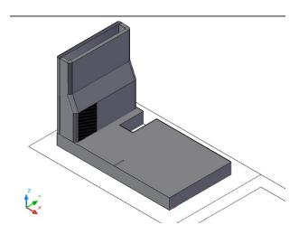
Left base channel. Cut a 6.75" wide opening as shown. (Not shown) also cut a cleanout opening on the right side, in line with the other cutout.
