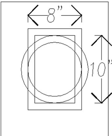
The cross sectional area of an 8" round is 50.25 sq.in. , and a typical 8x12 o.d. clay liner is around 6x10 inside, or 60 sq. in.
