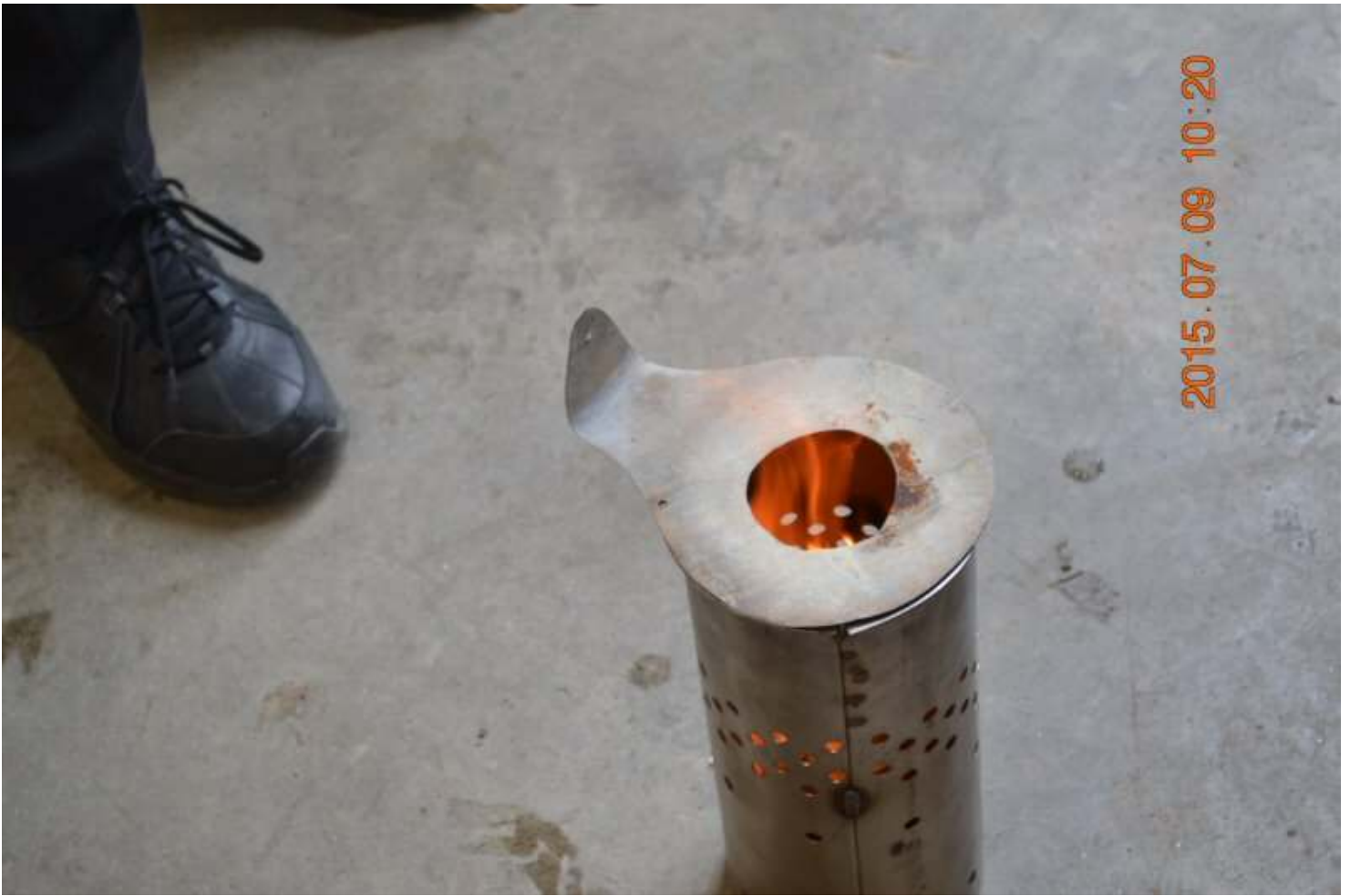
A restrictor to prevent cold air downdrafting in the tube.
