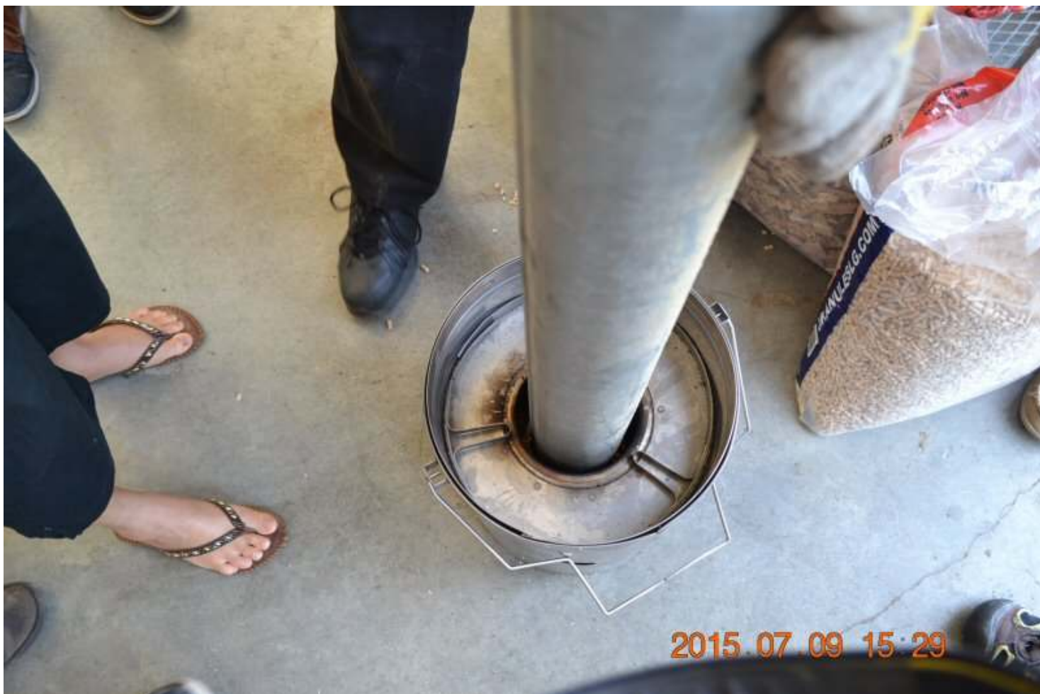
Lighting another TLUD stove, burning pellets. The 4" pipe is used to accelerate the draft and help get the pellets lit.
