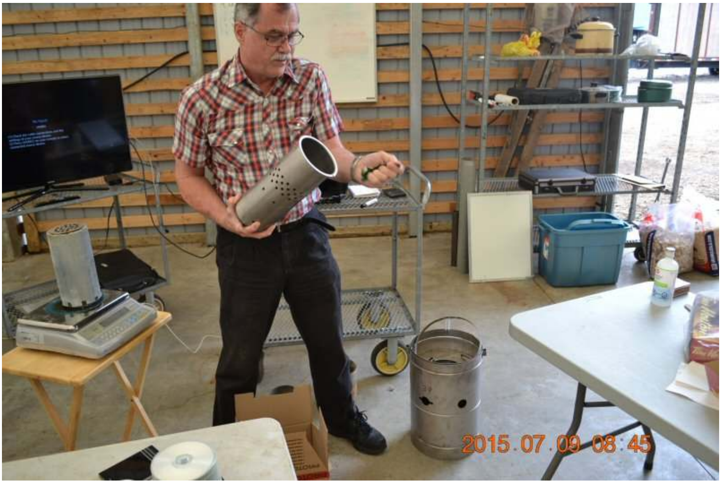
The burn chamber sits inside an outer sleeve that is used to preheat the secondary air.
