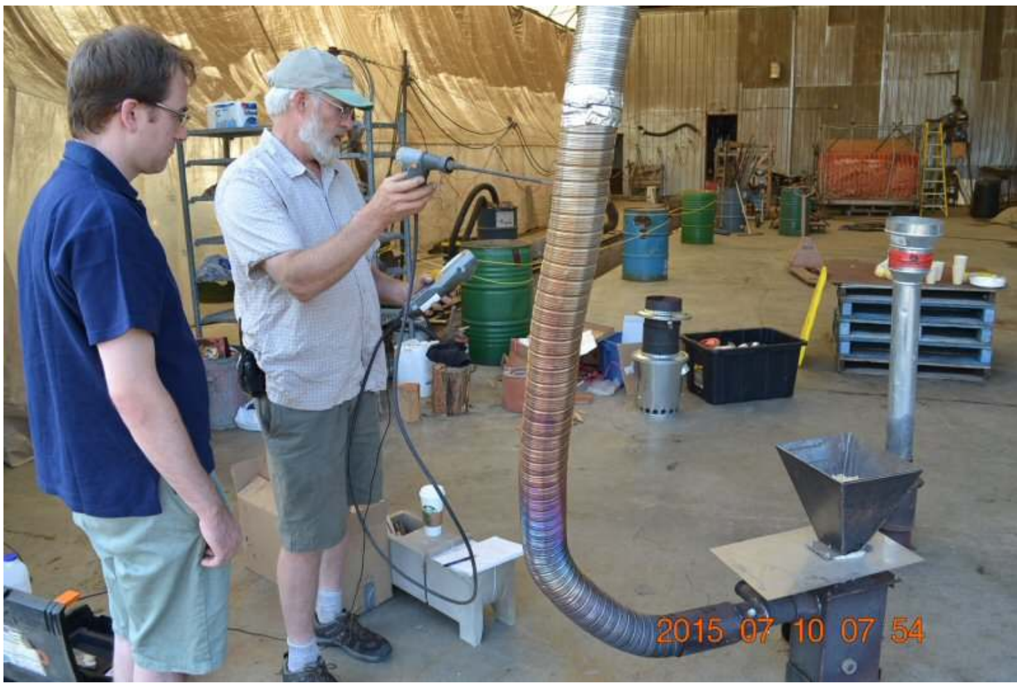
Checking the combustion with a Testo. It was very clean, with very low CO.
