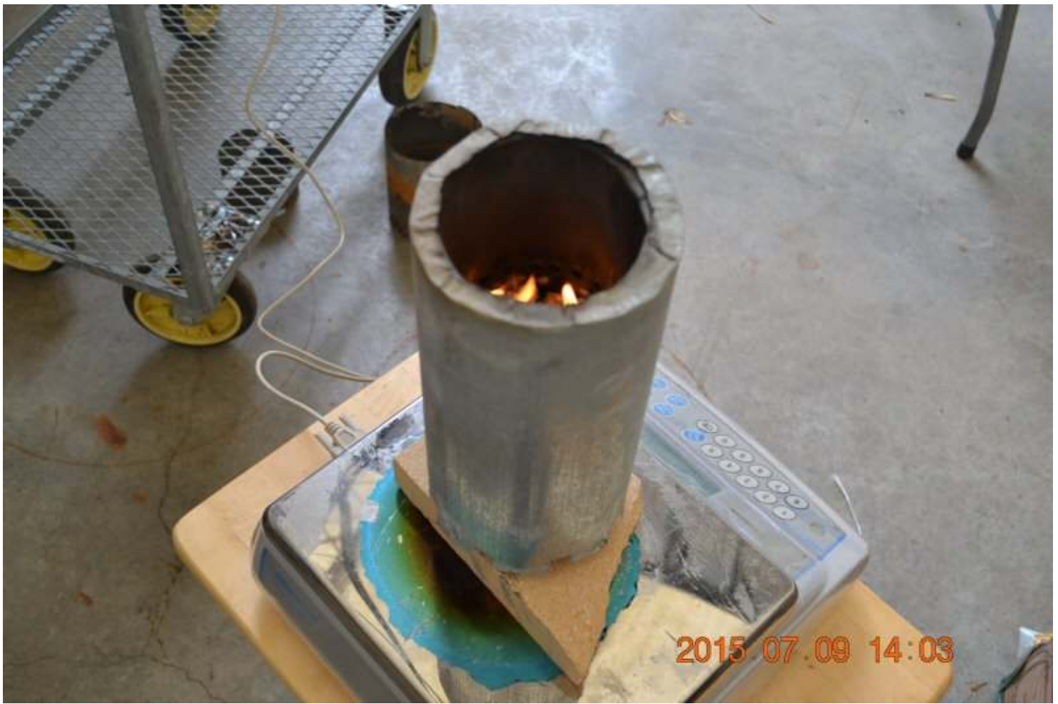
A $1.00 stove developed by Crispin for Haiti. It is sitting on a digital scale that measures the weight loss from the fuel in order to determine the burn rate and power output in real time.
