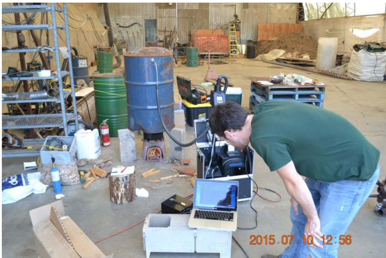
One of the participants, Rebecca Vermeer, is originally from Indonesia and does stove work there. Here we have her clay stove set up underneath an improvised hood using a steel drum. Note the hose from the Wohler sampler to the blue drum hood.
