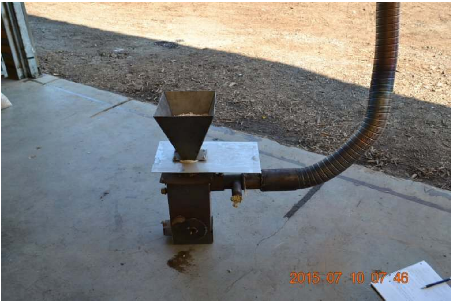
This is an experimental gravity feed pellet stove that Alex English built, and hooked up for a demo. It needs no electricity. The sprocket in the front is connected to a manually operated shaker grate.
