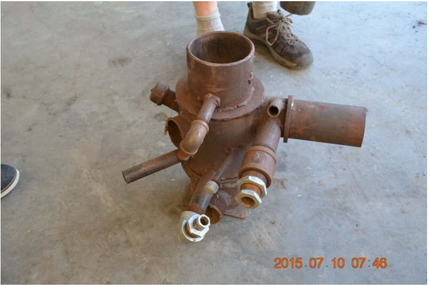
This is another prototype without a shaker grate.
