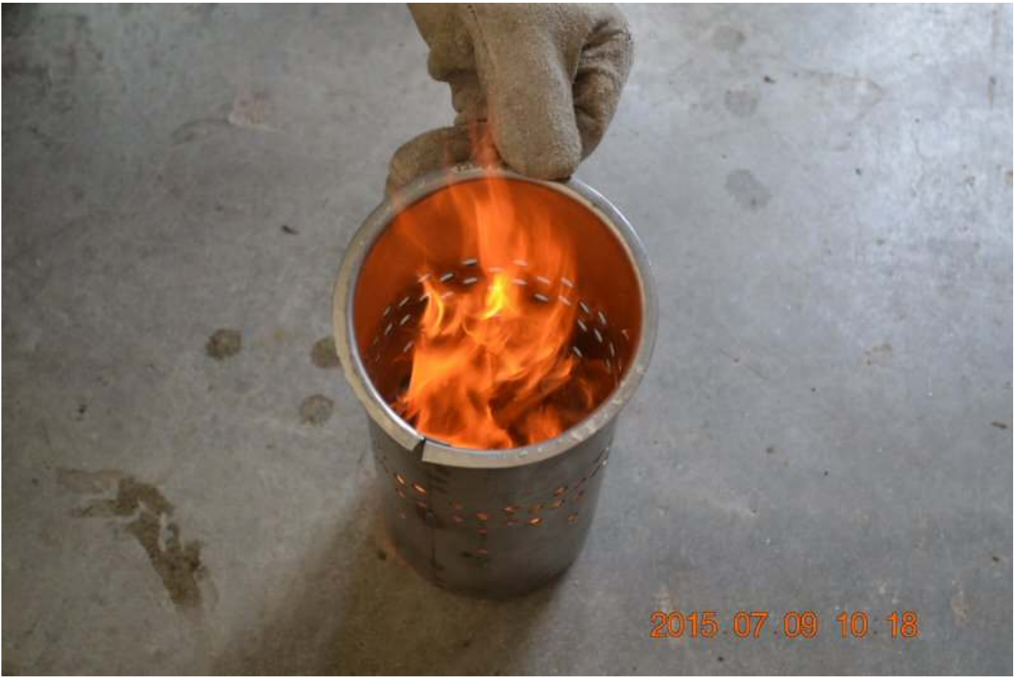
Secondary air holes at the top. Notice the initial long flaming of the wood gases.
