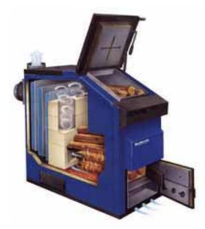
Figure 2-21 Under-burning boiler with induced draught, flue gas exit sideways(Buderus 2005)
