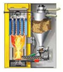
Figure 2-19 Horizontal feed boiler (*Hargassner 2005*)
