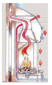
Figure 2-8 Functional principle of a log wood stove (Westfeuer 2005)
