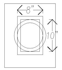
The cross sectional area of an 8" round is 50.25 sq.in., and a typical 8x12 o.d. clay liner is around 6x10 inside, or 60 sq. in.
